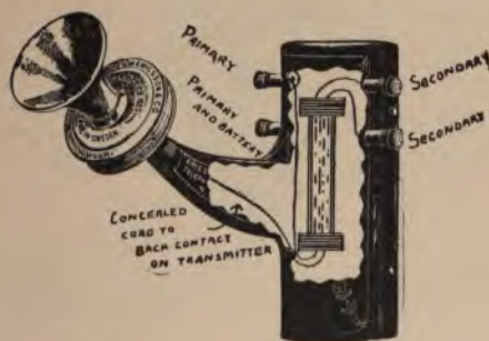
FIG. 8.—Section of transmitter arm and coil box, showing connections between the transmitter and induction coil.
